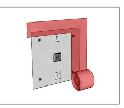
**5.** Cut and install the drywall around the fixture, ensuring that the fixture board assembly is flush with the surrounding drywall. This will allow a finish of one eight inch of plaster around the finishing guard.
