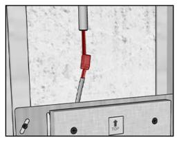
2. Feed low voltage wiring to the fixture board assembly and make the low voltage connection.
